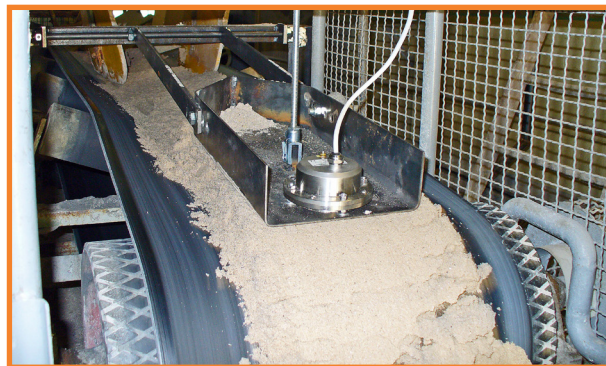
Measuring moisture of sand
