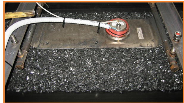
Measuring moisture of coal after the mill
