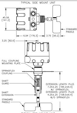
DIMENSIONS ARE SHOWN IN INCHES WITH MILLIMETER EQUIVALENT IN BRACKETS
