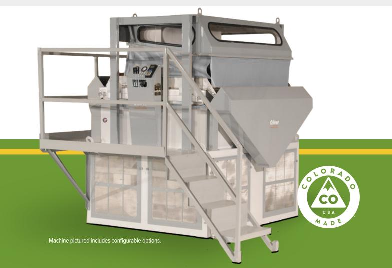
This maximum capacity destoner purifies your product by separating heavy materials such as glass, dirt, stones and metals from larger quantities of lighter material. Add value on a variety of products with the most precise destoner on the market – Oliver's legendary Maxi-Cap Destoner.
